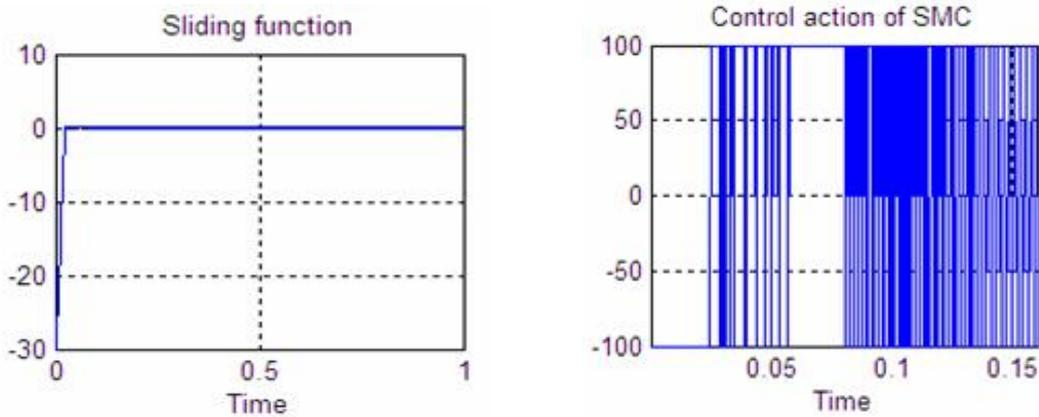
Figure 2: The responses of the DC motor system (18) using the SMC (20) without disturbance.
