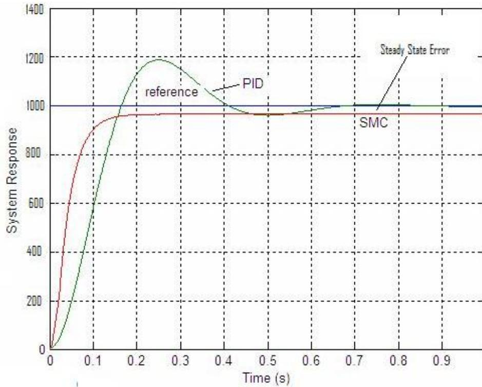
Figure 3: The output response for the DC motor without disturbance using PID controller and SMC.
