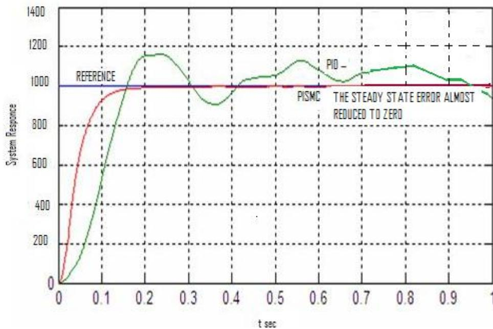
Figure 4: The responses of the DC motor system with disturbance using PID and PI - Sliding mode controllers.
