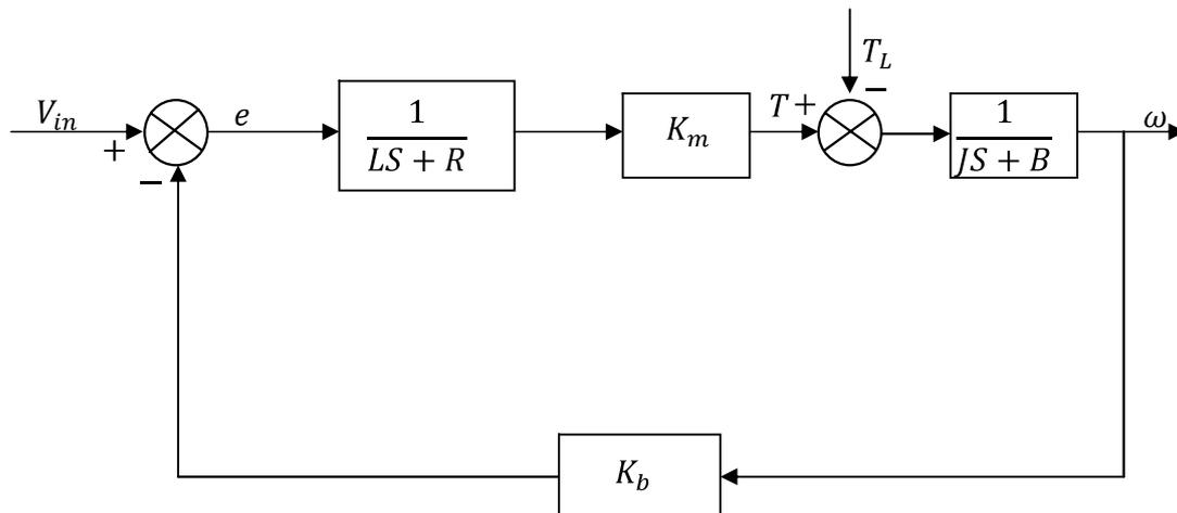
Fig 1: Block Diagram of BLDC motor
