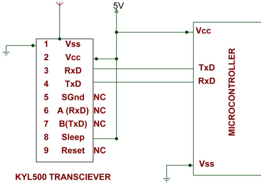
Fig 4: RF Transceiver Circuit Diagram
