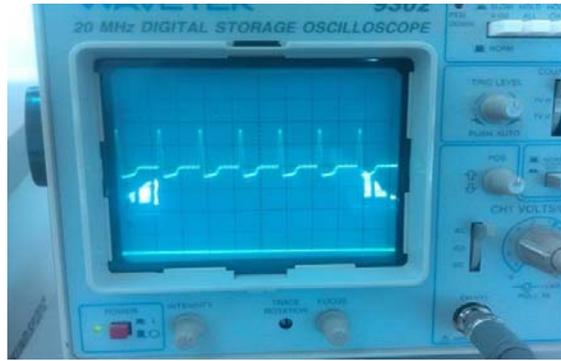
Fig 13a Operational amplifier output waveform at 3.333kHz and peak voltage 2V
