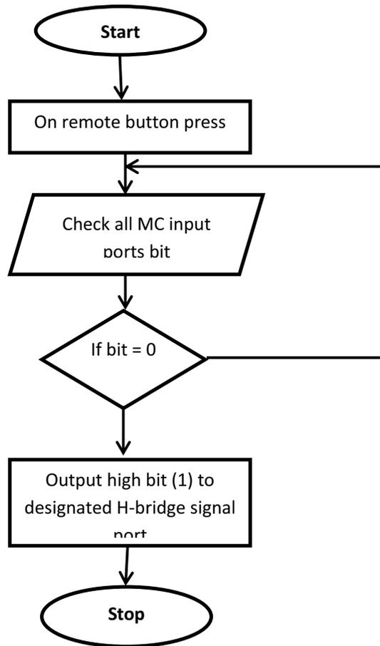
Fig 6: Wheel Control Flow Chart
