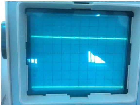
Fig 12 Voltage divider output DC wave form at 1.8V
