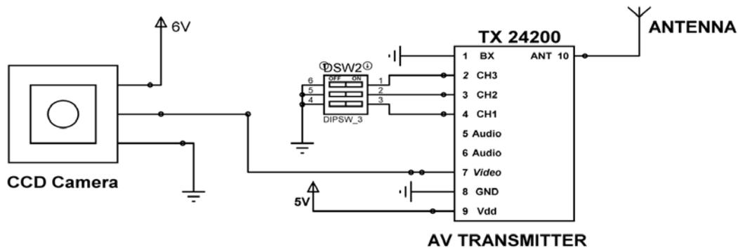
Fig 2 CCD Camera to Video Transmitter Module Circuit Diagram
