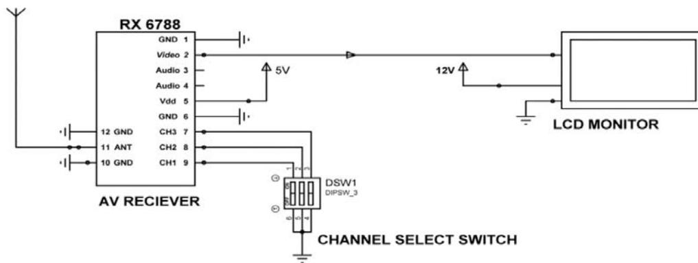
Fig 3: Video Receiver module to Monitor Circuit Diagram
