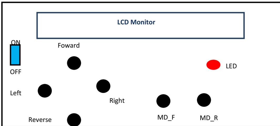
Fig 5: Control Buttons Arrangement for the handheld device
