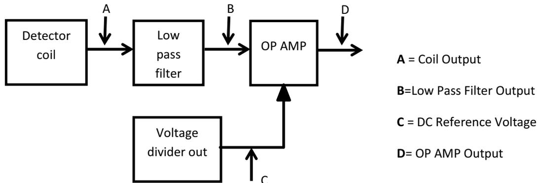
Fig 9 Voltage and Frequency Test Points
