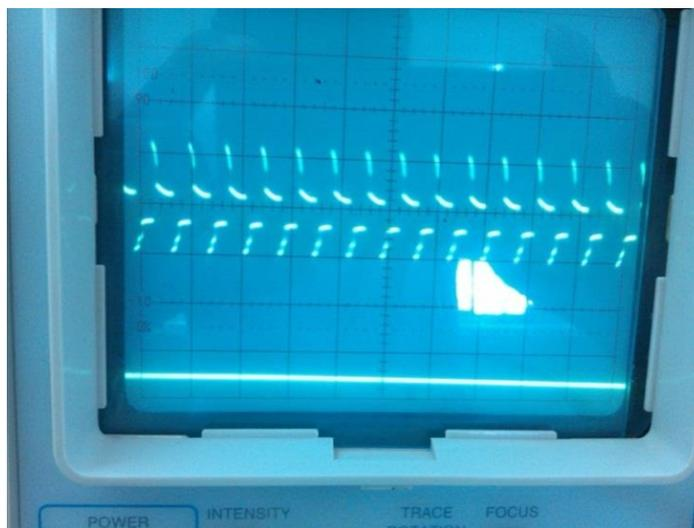
Fig 10c Coil Waveform In the Presence of a Non-ferrous Metal at 3.57 kHz
