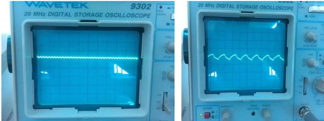
Fig 11a Rippled DC output of low pass filter at 1.95V
