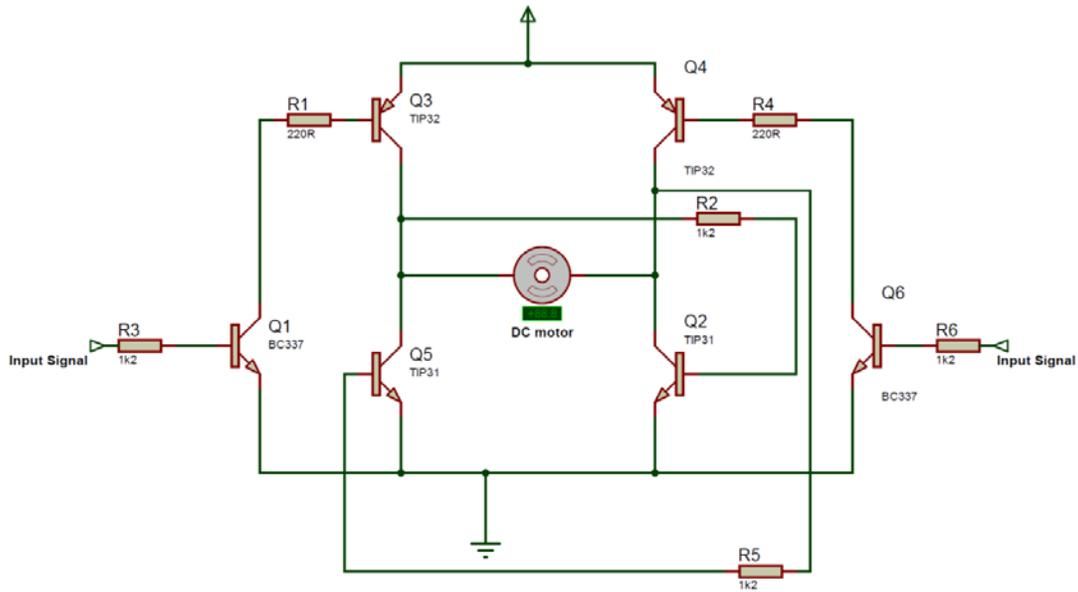
Fig 1 Complete full H-bridge circuit Diagram.
