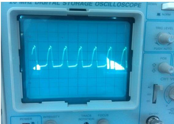
Fig 13c Operational Amplifier output at 3.700 kHz in the presence of non-ferrous metal
