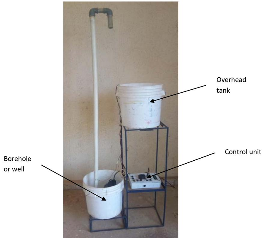
Figure 3: Setup of proposed domestic water control system
