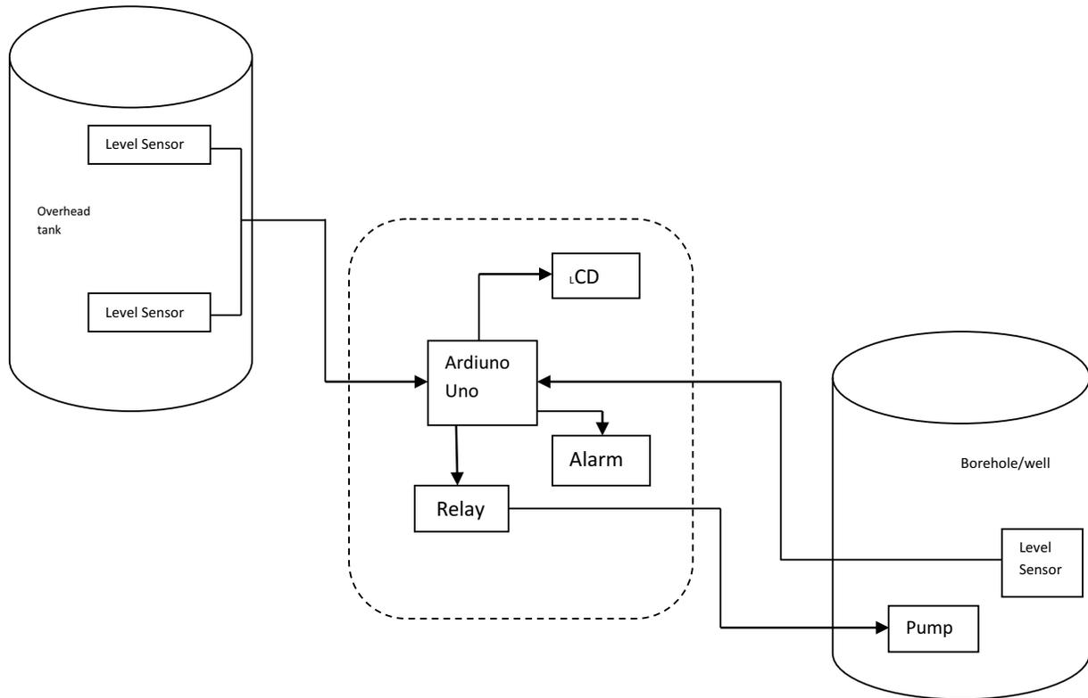
Figure 1: Block diagram of Automated Domestic Water Control System
